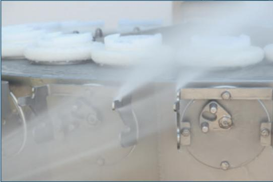
The actuators are turned and therefore offers a smoother surface. An angled top fully welded onto the sleek body, leads to no unhygienic edges or overlapping seams. Under the principle of "fix only what is broken", you can access or replace individual components. One actuator eg comes free by loosening just 4 bolts. This is part of the reason why this machine is the most economic machine to maintain on the market.
