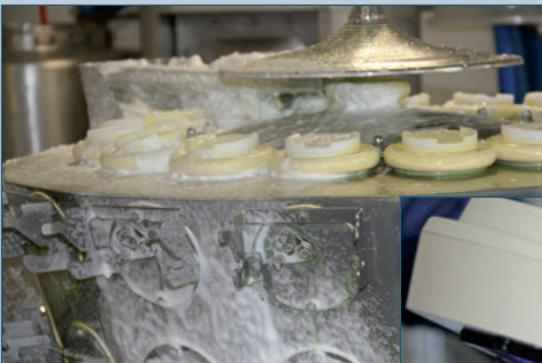
Every tiny detail has been carefully designed for highest level of hygienic design and best sanitation. The machine has gone thru and passed all of the toughest bacterial tests. As part of the tests, a hand-held device scans for potential bacterial leftovers after sanitation.
